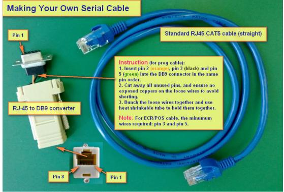
b. Below is the pin mapping between the DB9 and RJ45
